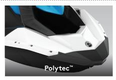
Innovative material that reduces weight while optimizing performance and efficiency. The color-in molding is more scratch-resistant than fiberglass.
