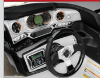
Premium helm with Cruise control, Ski mode (twin engine only) and ECO™ mode
